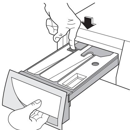
Flush it out under a tap, to remove any traces of accumulated powder.
